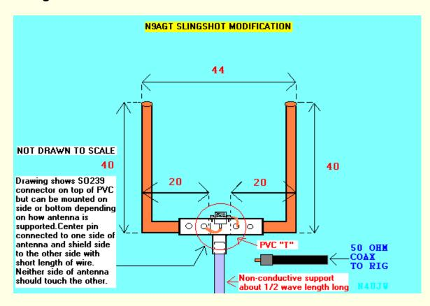
To make the connections to the 239 connector, I bore oversized holes into the PVC so that the screw head and nuts would contact the copper tubing. I bought the brass screws long enough -  $1 \frac{1}{4}$ " - so that I could put two nuts on them; one to hold it to the tubing and the other to act as a lug to connect a short piece of bare #14 copper wire to. I then soldered the other end to the 239 connector. I repeated that for the other side. This makes it a neat and clean antenna.
